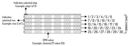
> Select DMX channel with < V > button and select DMX value with the fader corresponding to the DMX channel,
