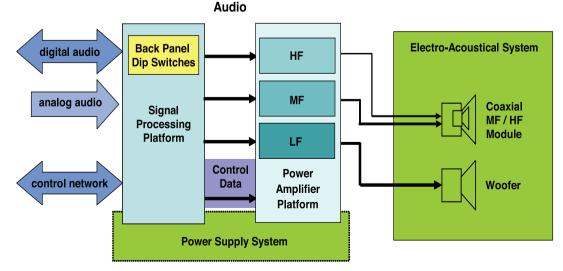
Figure 3: Main building blocks of Genelec 8260A loudspeaker.
