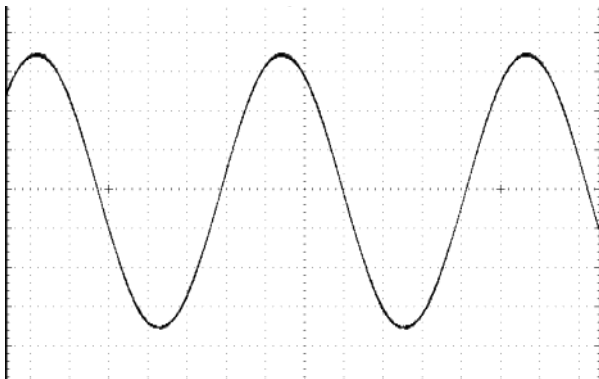
This trace shows two signals, one running through the drive circuit and one not. As the clip threshold has not been reached, both signals are identical.
