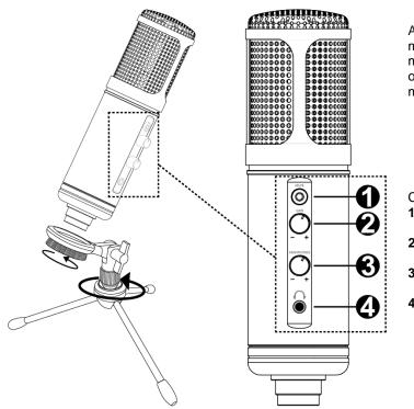
Attach the microphone holder to the tripod by turning the mounting ring counter-clockwise. Repeat to mount the microphone in the microphone holder: turn the mounting ring of the microphone holder counter-clockwise to fasten the microphone securely.
