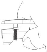
2 Remove the cartridge in the direction of the arrow while holding the stylus holder part with your other hand.
