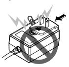
When mounting the AC adapter on a wall outlet, make sure there is no space between the AC adapter and the wall outlet. Faulty contact or a coin, paper clip or other metal object getting stuck in the space could cause a short circuit, leading to fire or electric shock.
