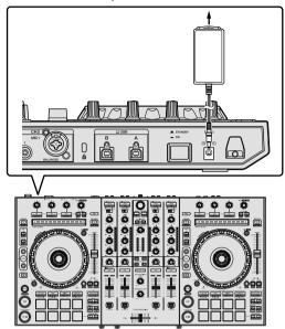
7 Press the [ $\circlearrowleft$  STANDBY/ON] switch on this unit's rear panel to turn on this unit.
