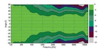
Figure 5: Horizontal directivity plot of Genelec 8260A.
