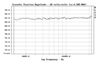
Figure 4: On axis frequency response of the Genelec MDC driver. The frequency response shown is from 2 kHz to 20 kHz.
