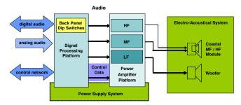
Figure 7: Main building blocks of Genelec 8260A loudspeaker
