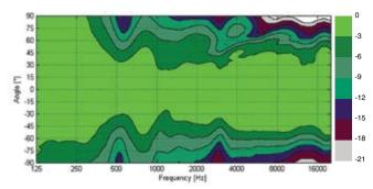
Figure 6: Vertical directivity plot of Genelec 8260A.
