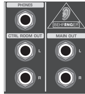
Fig. 2.9: Monitor/main mix connectors
