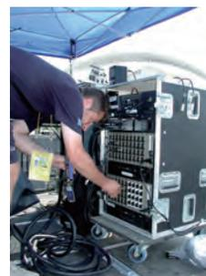
◀ A picture of the customized setup using a rack mounted S-4000S I/O module
