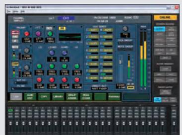
M-400RCS remote control software. You can setup configurations and channels ahead of time, save existing projects and adjust any type of mixer setting, recall scenes, load presets, etc.
