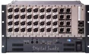
32 in/8 out for stage use. All inputs have remote preamp/PAD/phantom power. 24-bit/96kHz AD/DA converters. Audio transmission and power supply redundancy.
