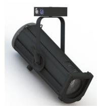
The PLFRESNEL-1 is a general purpose luminaire for theatre, small studio, and display lighting applications which produces an adjustable cone of light with a soft edge which is easily blended with adjacent beams to provide even illumination. Using LED source technology combined with a traditional Fresnel lens, the **PLFRESNEL-1 delivers Philips** Selecons industry benchmark quality without the compromising performance of spreader lenses.
