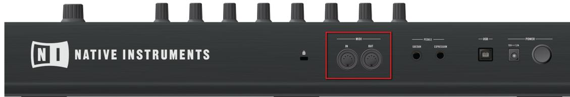
MIDI ports on the back of the KOMPLETE KONTROL S-SERIES keyboard
