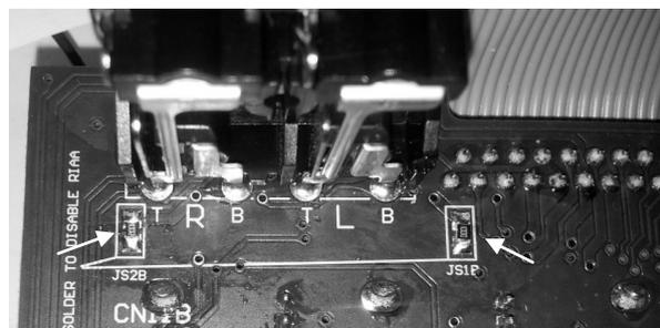
If the RIAA input level is too low, or you wish to convert them to Line level. To increase the gain by 6dB, remove the resistors arrowed and link the Pads with solder. These resistors are located on the underside of the front panel PCB, directly behind the Input RCA connectors
