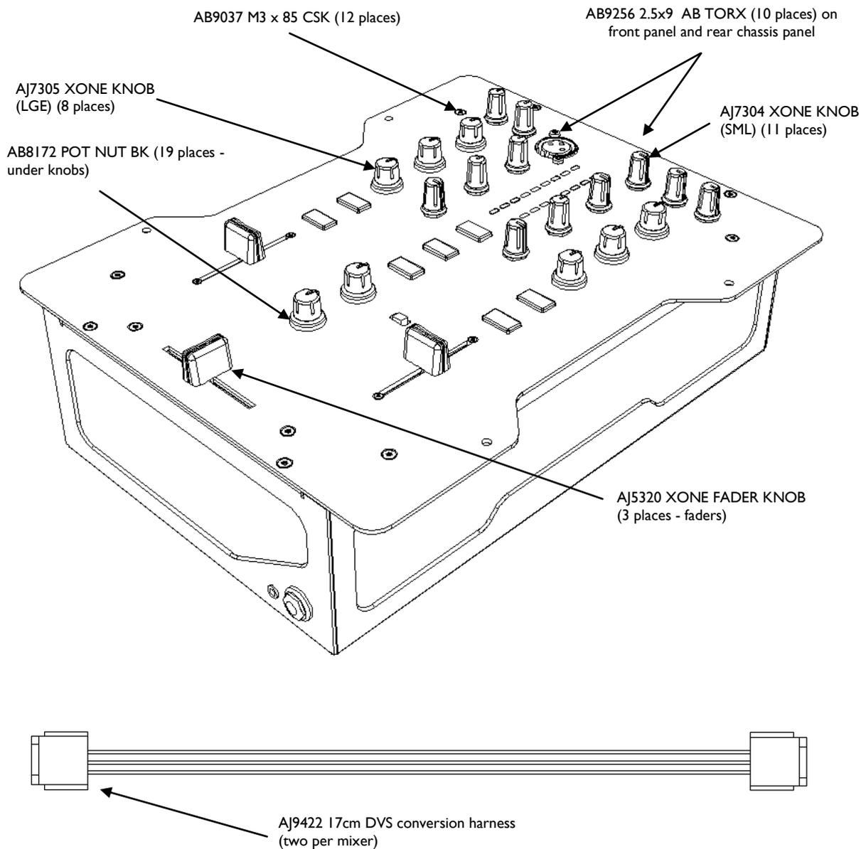
The diagram above shows all of the replacement parts that can be ordered from your local technical support, or direct from Allen & Heath, for the Xone:23C. When ordering please quote the part number(s) of the required parts.
