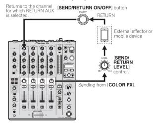
[INSERT]: The audio of the channel selected in the effects channel is input to the external effector (or mobile device), and the output from the external effector (or mobile device) is input into the channel selected in effect channel.
