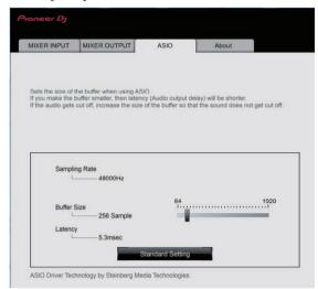
If a large buffer size is set, drops in audio data (breaks in the sound) occur less easily, but the time lag due to the delay in the transfer of the audio data (latency) increases.
