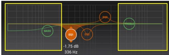
User Peaking EQ Controls: Center Frequency, Q, and Gain parameters are controllable for these three.
