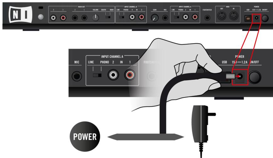
We strongly recommend you to use an external power supply with your S4 via the included power supply unit. Although operation is also possible when your S4 is powered via the USB connection, you then have following limitations: the headphones output level is lower, and all LEDs light darker. Moreover, your device might then be subject to USB power-related issues, as explained in section [↑9.2.4, USB-related Power Issues](#).
