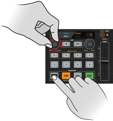
Holding SHIFT + turning the MOVE encoder to adjust TRAKTOR DJ's viewing scale.
