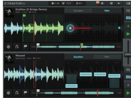
Turning Channel A's FILTER anti-clockwise to initiate a LFP Filter, and the corresponding Filter movement along the X Axis in TARKTOR DJ.
