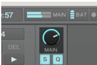
If you see some activity on the **MAIN LEVEL** meters of your S4 but don't hear any sound, then double-check the connection starting with the cable going from the S4's Main Outputs to your PA.
