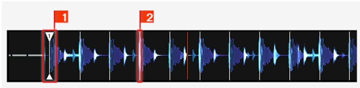
A track's waveform with Grid Marker (1) and the Beatgrid (indicated by the white vertical segments, 2).
