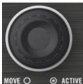
3. Turn the Loop **MOVE** encoder to select the **All Remix Sets** folder from the Browser Tree. Press the Loop **MOVE** encoder button to expand the folder node.
