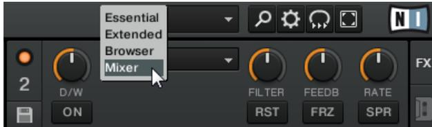
To change the Deck Flavors, click on the Deck letter in a Deck's upper right corner and select a Flavor from the drop-down menu:
