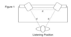
**Mid-Field Configuration:** This configuration is essentially the same as the Close-Field setup (see Figure 2). The Mid-Field configuration is normally used with larger monitors or when the monitors are too large or heavy for the meter bridge, as is likely the case with the Exposé E8B. This set-up has the potential for a larger sweet spot and better spatial imaging. Ensure that the height of the woofer is above the height of the console's meter bridge.
